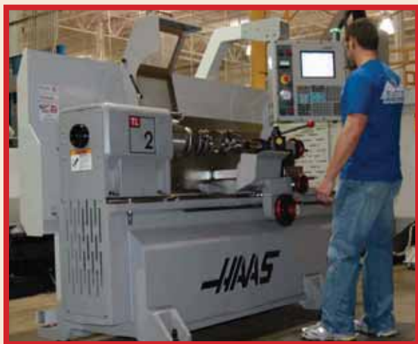
Crankshaft rear flange being machined on Haas CNC lathe to ensure a precision fit of flex plate or flywheel.
